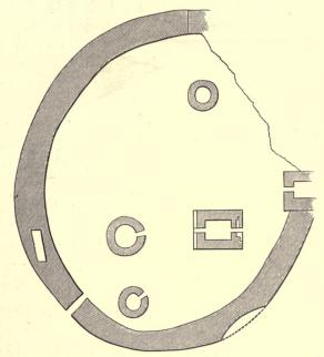
Fig. 32.—Ground-plan of the Cashel and its included structures on Oilen-Tsenach. (From Lord Dunraven's Notes on Irish Architecture.)
